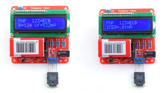
Display the Collector cutoff current Iceo with currentless base (10uA units) and Collector residual current Ices with base hold to emitter level. This values are only shown, if they are not zero (especially for Germanium transistors).
